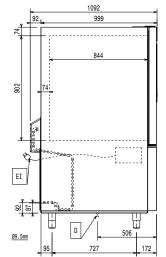
Drain Electrical inlet (power) FΙ Refrigerant Outlet
